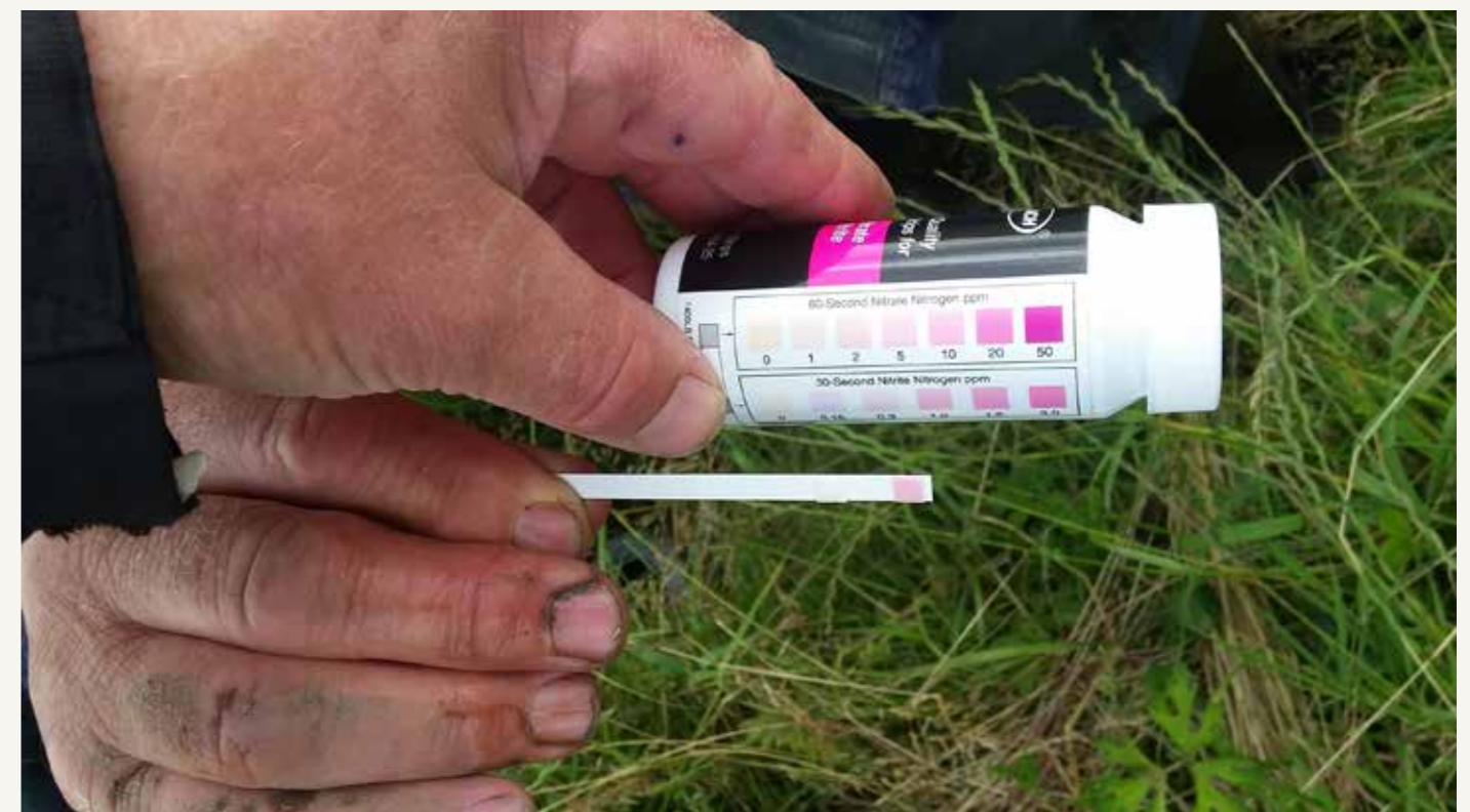
Test strips are practical for deciding levels of nitrate concentration.
