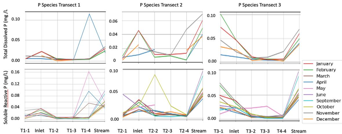
**Figure 8.** Total phosphorus and phosphate as monthly mean concentrations in in the three transects of the saturated buffer zones, in the inlet and in the stream. The first transect point represent the shallow groundwater before of the distribution pipe, the inlet represents the drain water, and the stream was sampled upstream before the saturated buffer zone.
