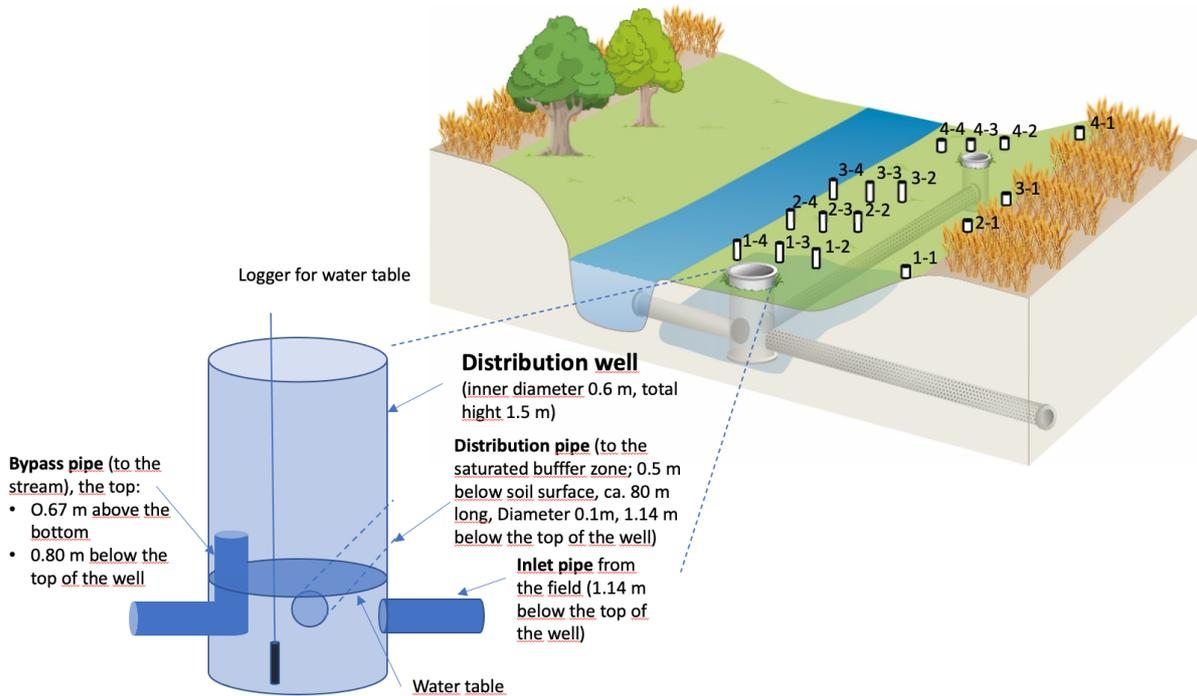
**Figure 2.** Layout of the instrumented saturated buffer zone (SBZ). Three transects with piezometer are in the SBZ and one control transect (4-1, ..., 4-4) in a natural wetter part of the riparian zone.
