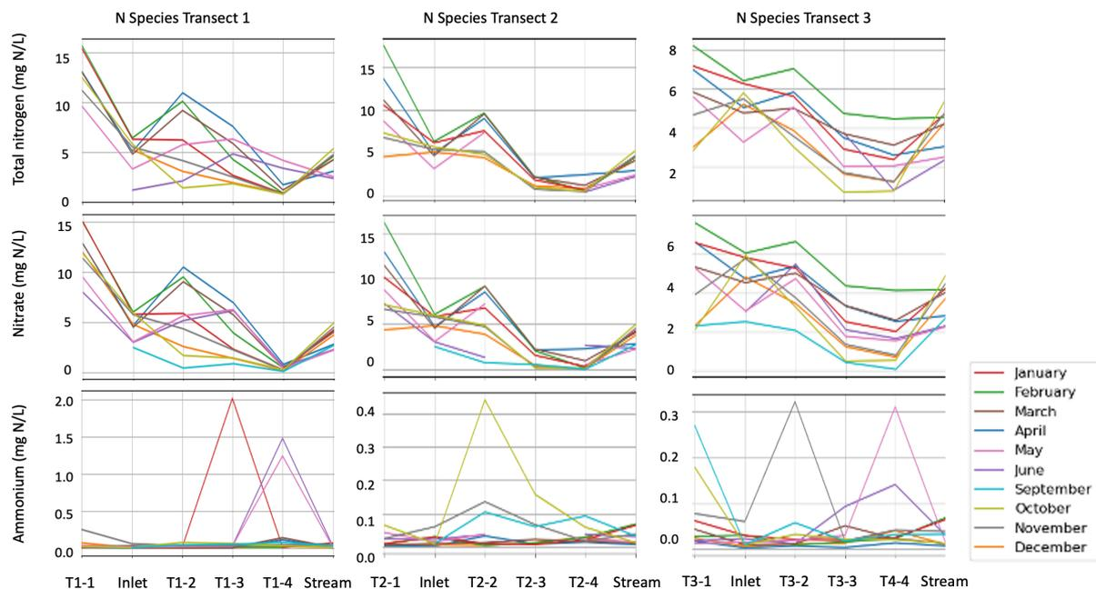
**Figure 7.** Total nitrogen (TN), nitrate and ammonium as monthly mean concentrations in the three transects of the saturated buffer zones, in the inlet and in the stream. The first transect point represent the shallow groundwater before of the distribution pipe, the inlet represents the drain water, and the stream was sampled upstream before the saturated buffer zone.
