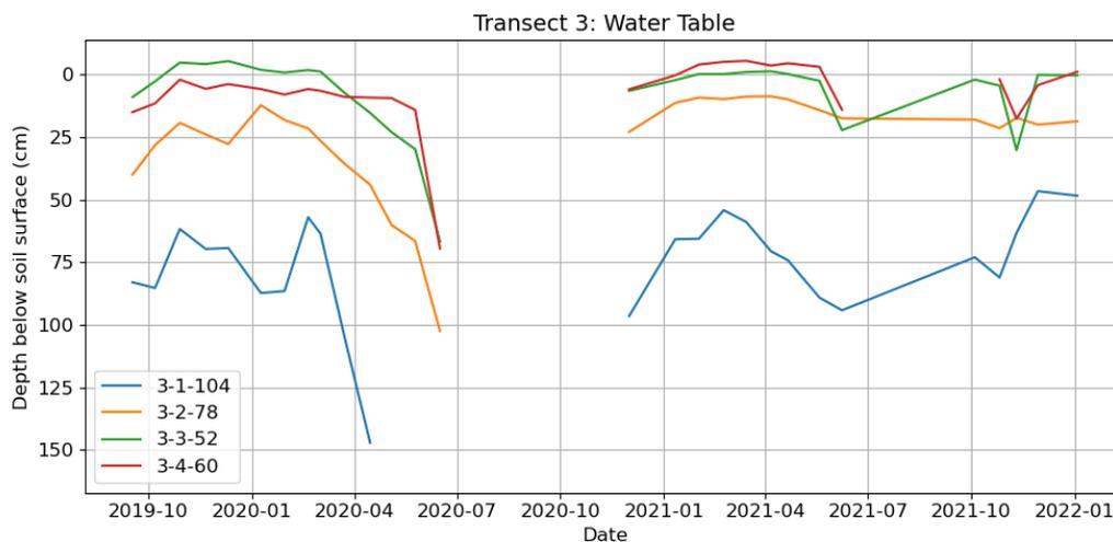
**Figure 6.** Temporal changes of water tables in relation to the soil surface in transect 3. The first point (3-1-104) is located at the edge of field (see Figure 2) not influenced by the drain water but by shallow groundwater
