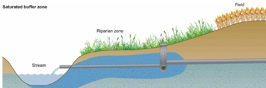
**Figure 1.** Conceptual scheme of a saturated buffer zone. The drainage pipe is diverted into a distribution pipe charging the SBZ until water saturation depending on the amount of infiltrating water during the year. Surplus of water is directed to the stream over a vertical bypass pipe in the distribution well presenting the old drainpipe (image from Carstensen et al. 2020)
