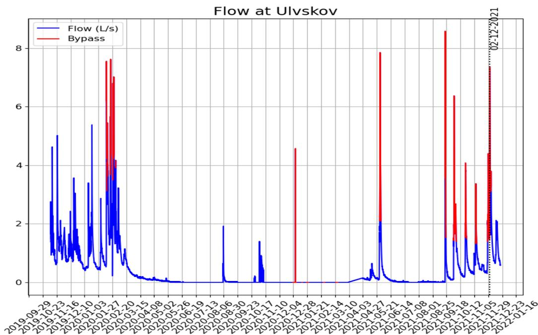
**Figure 4.** Flow and bypass flow for Ulvskov for the entire project period. The blue line shows the flow, while the red indicates when bypass flow has occurred. The dashed line shows the date (02-12-2021) when the distribution pipe was rinsed to decrease bypass flow.
