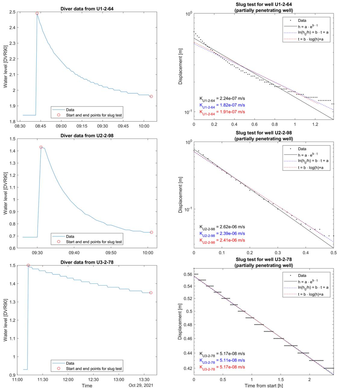
**Figure 5.** Demand of time for water tables to decrease after water addition (slug tests) to determine the hydraulic conductivity (HYC) in the middle of the saturated buffer zones: piezometer points 1-2, 2-2, 3-2 (left column). Different models were applied for calculating the HYC (right column).
